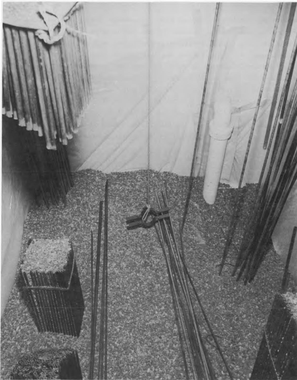
Figure 16. Chamber for systems operations test. The sump below the former SPERT-II reactor is shown after installation of test targets and before filling with water. Fuel bundles and individual fuel rods on the floor and stacked in the corner of the pit are mocked up with small-diameter tubing and pipe. Crushed gravel on the floor and the tops of fuel bundles mock up known debris. The pit measured 2.44 x 2.44 x 1.8 m. (EG&G Idaho photo 83-6-2-9.)
